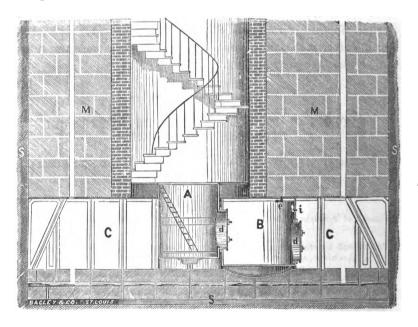
The caisson, C C, upon which the solid masonry, M M rests is octagonal in shape, eighty feet long, forty-five feet wide, and
