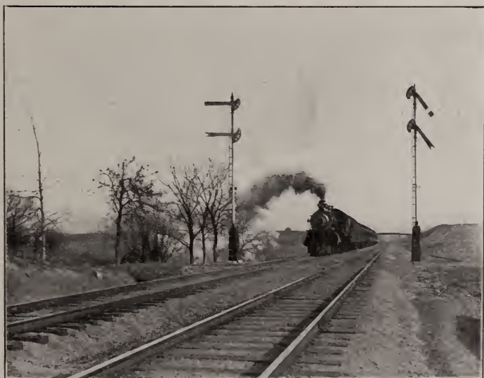
The Lo: Angeles Limited on the Union Pacific, Obeying "Stop" Signal on Lane Cutoff, near Omaha, Nebraska.
