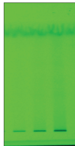
Figure 6: High-performance thin layer chromatography video image of Erigeron canadensis at 254 nm in chloroform: methanol (9:1 v/v)
