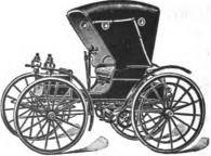
The Holsman is air-cooled, has solid rubber tires and is built high enough to clear country roads like a carriage.
