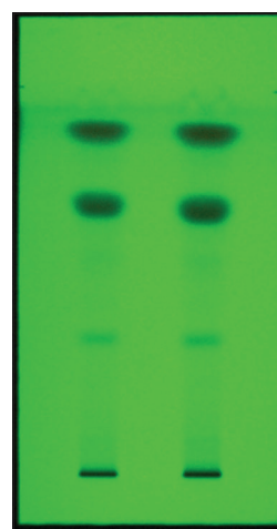
Figure 5: High-performance thin layer chromatography image of Rumex crispus at 254 nm in hexane: Ethyl acetate (6:4 v/v)
